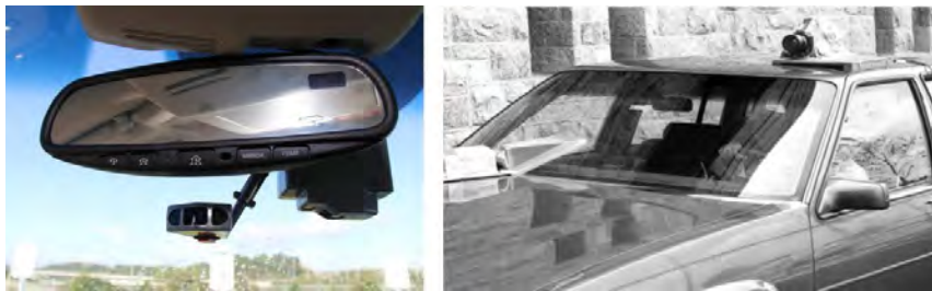
Early transportation research instrumentation, which became the basis for the VTTI naturalistic driving study research method (left). Newer instrumentation that captures a view of the driver's face, which can tell us a lot about driver behavior in the real world (right).
