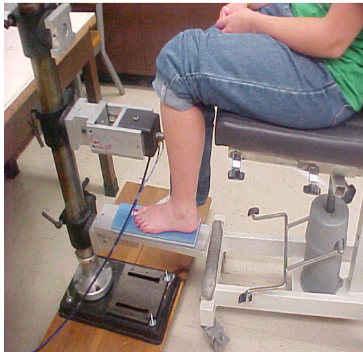
Figure 1.6: Current MRTA experimental system for tibia strength assessments (reproduced with permission: Herbert, 2004)
