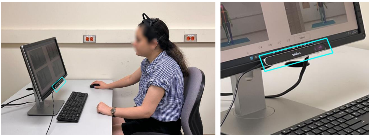
Figure 2.4 Experiment setup with a monitor equipped with a screen-mounted eye-tracking device.
