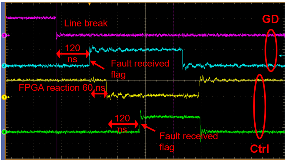
Figure 39: Fault recognition timing waveforms
