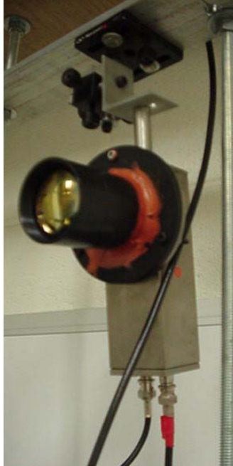
Figure 3.17. OH* Chemiluminescence Receiving Optics – Turbulent Combustor. The turbulent combustor used a lens and filter system.
