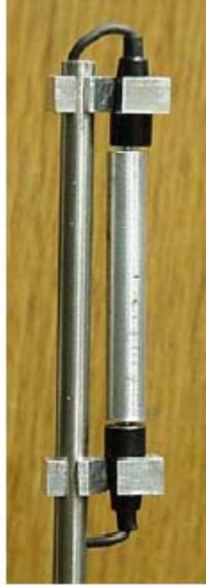
Figure 3.18. Velocity Sensor used in the Laminar Burner. The sensor is located directly upstream of the honeycomb.
