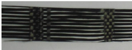
Figure 2.4: Sample used in resistive heating tests for thermal imaging.
