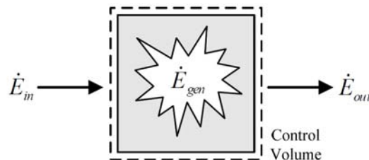
Fig. 2-4. Energy flow through a control volume
