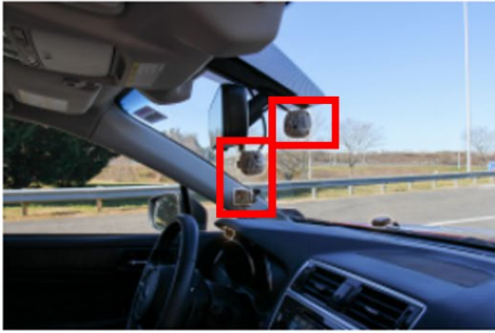
Interior camera installations and Incident Button Box
