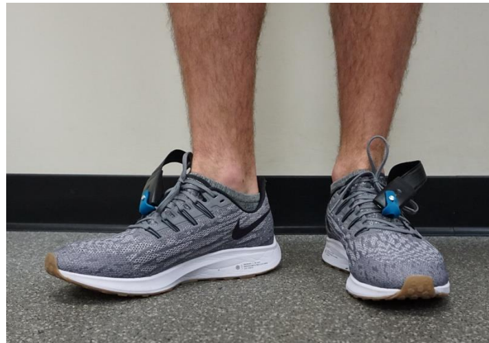
Figure 19 loadsol ® sensor inserted in standardized shoes
