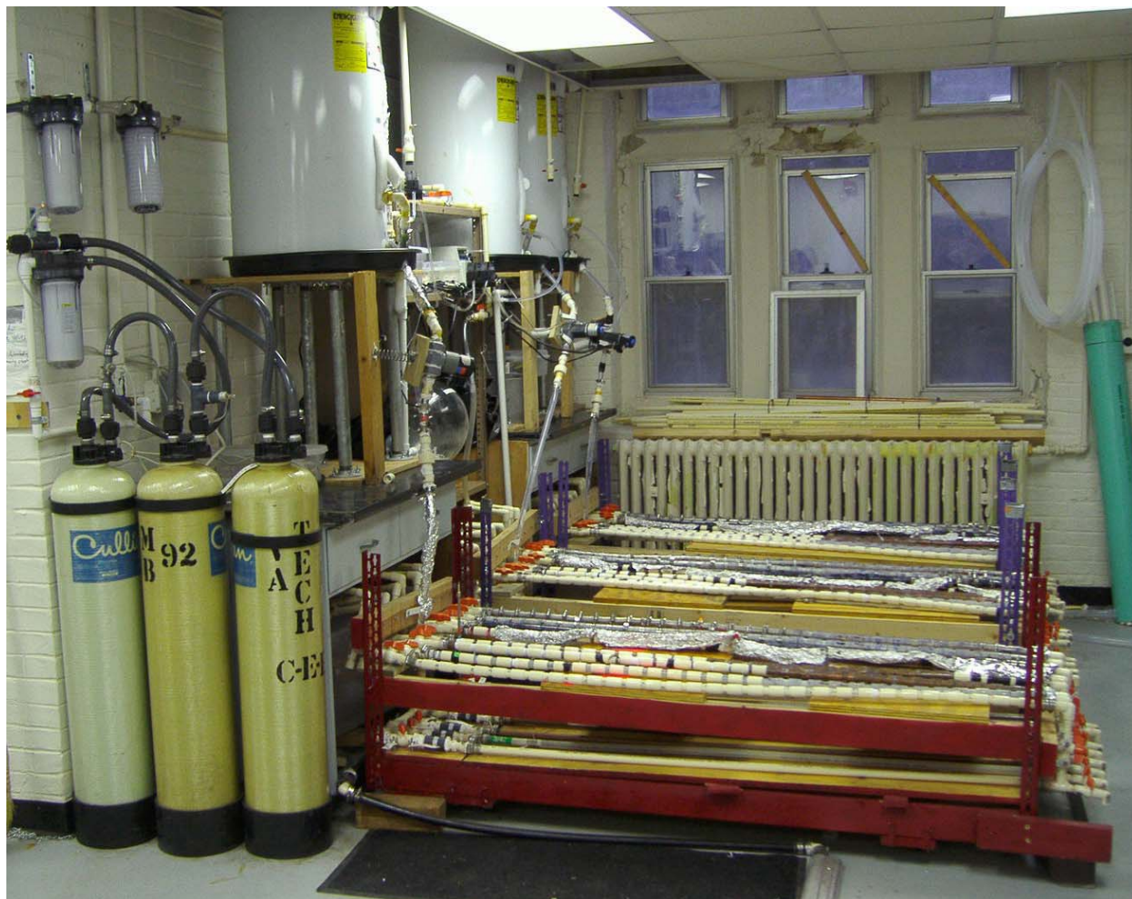
Figure 4-1. Simulated plumbing rig systems.
