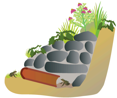
Figure 18-5: Rock pile habitat with large opening on bottom to allow amphibians to enter.
