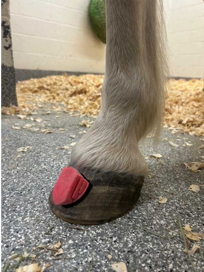
Figure 3.1 Image of a hoof-mounted inertial measuring unit affixed to the midline on the dorsal aspect of the hoof wall approximately 1 cm distal to the coronary band.
