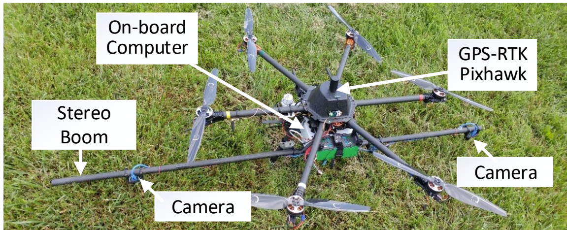
Figure 7: Stereo rig mounted on hexacopter
