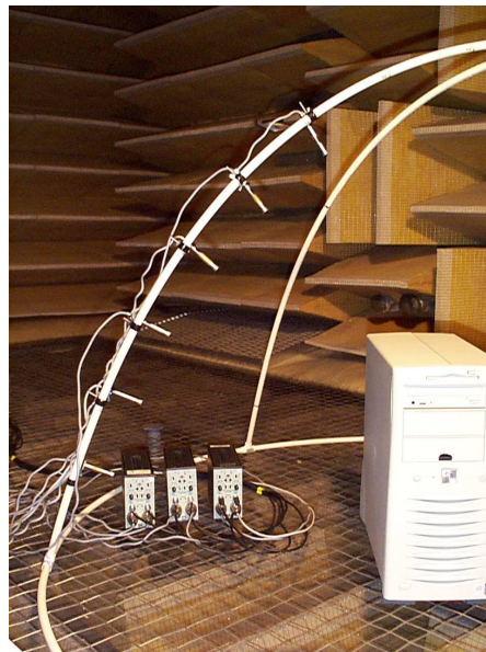
Figure 3.22 Directivity measurements in a VAL anechoic chamber.
