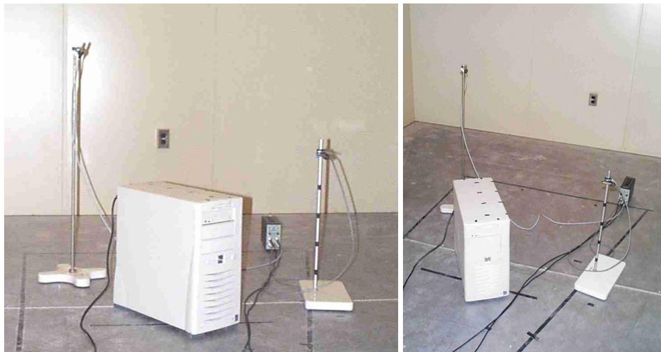
Figure 2.3 Sound power level measurement in one of the VAL reverberation chambers
