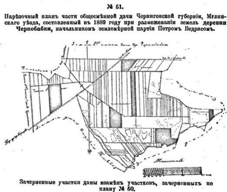
Figure 7 – Plan of the village Chernobabka of Chernygov governorate. Upper image shows the plan of the commune, while lower image shows a proposed plan for enclosure, drawn by a head of the surveying company Pyotr Vedris. (Source: Kofod 1906, 94)
