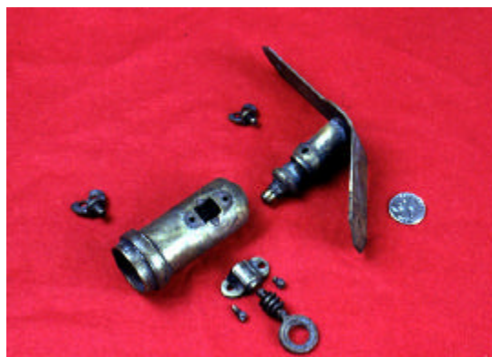
Figure 1.8: Universal staff mount made of brass
