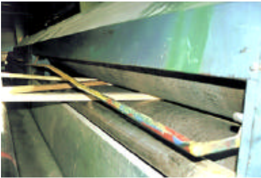
Fig 51: Truss is pressed in roller
