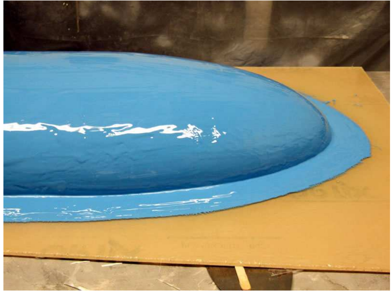
Figure 2.8: Mold epoxy surface coat
