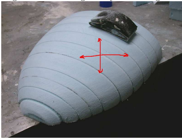
Figure 2.3: Sanding the curved surface
