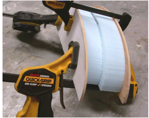
Figure 2.2: Gluing segments together
