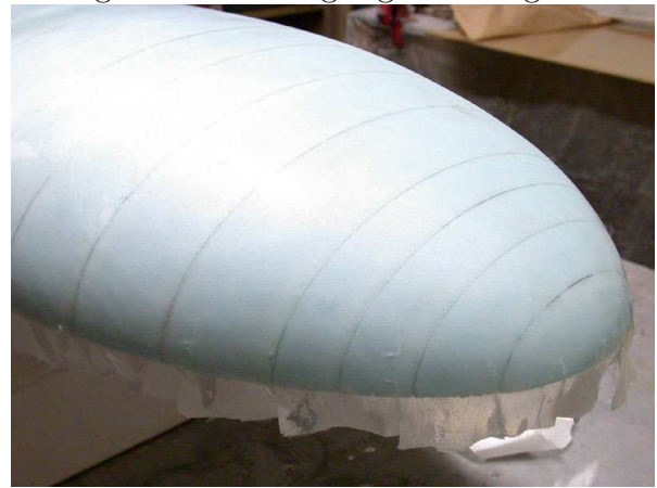
Figure 2.4: Reinforcing the surface with fiberglass cloth and epoxy
