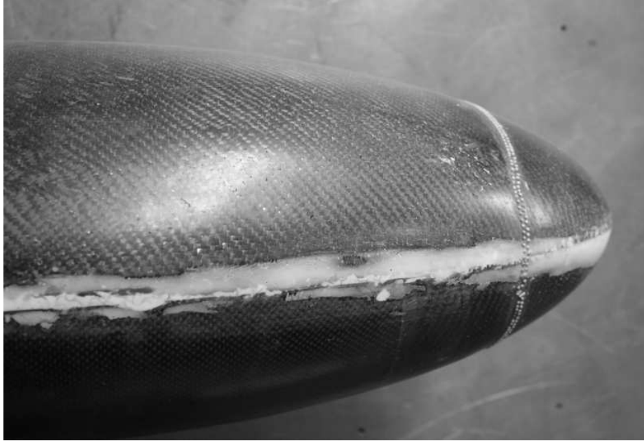
Figure 2.15: Boundary layer trip location on the model bow
