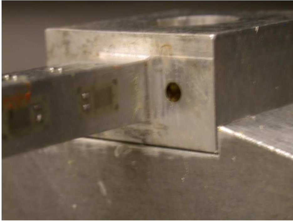
Figure 2.26: New style loadcell mount with ramp integrated in ring
