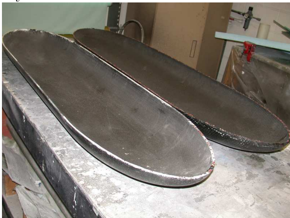
Figure 2.9: Layers of fiberglass cloth plus 2" Styrofoam stiffeners
