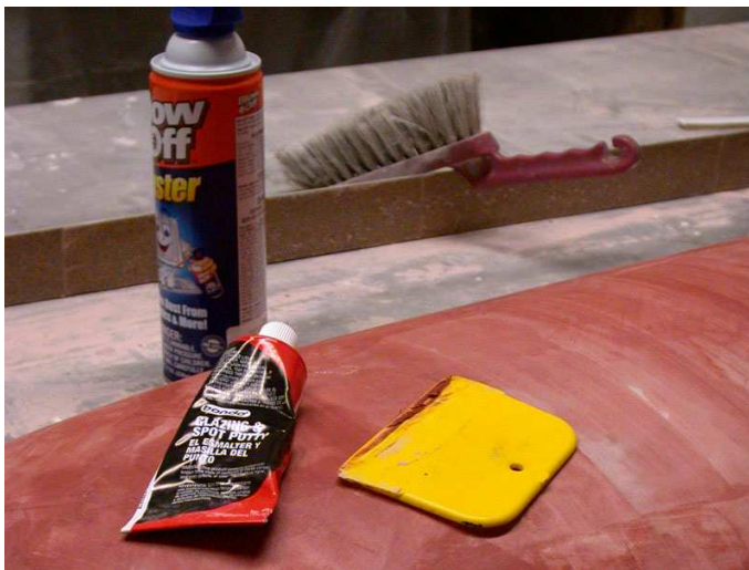
Figure 2.5: Smoothing the surface with spot putty
