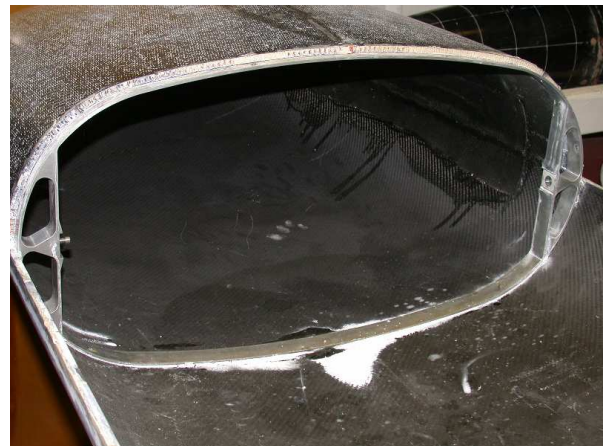
Figure 2.12: Aluminum ring inserted
