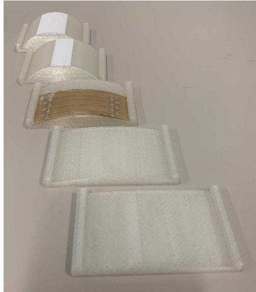
Figure 2.16 Composite sample holders with decreasing radius of curvatures, measuring from bottom to top: 635mm, 317.5mm, 158.75mm, 80.65mm, and 69.85mm.
