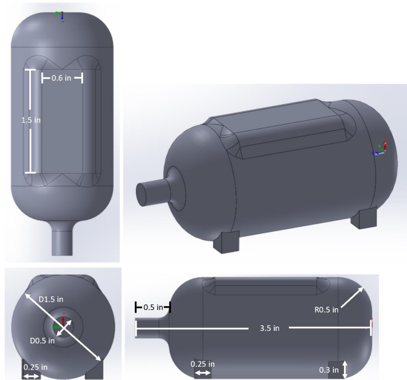
Figure A.2.1 Pressure vessel dimensions for FDM printed sacrificial tooling
