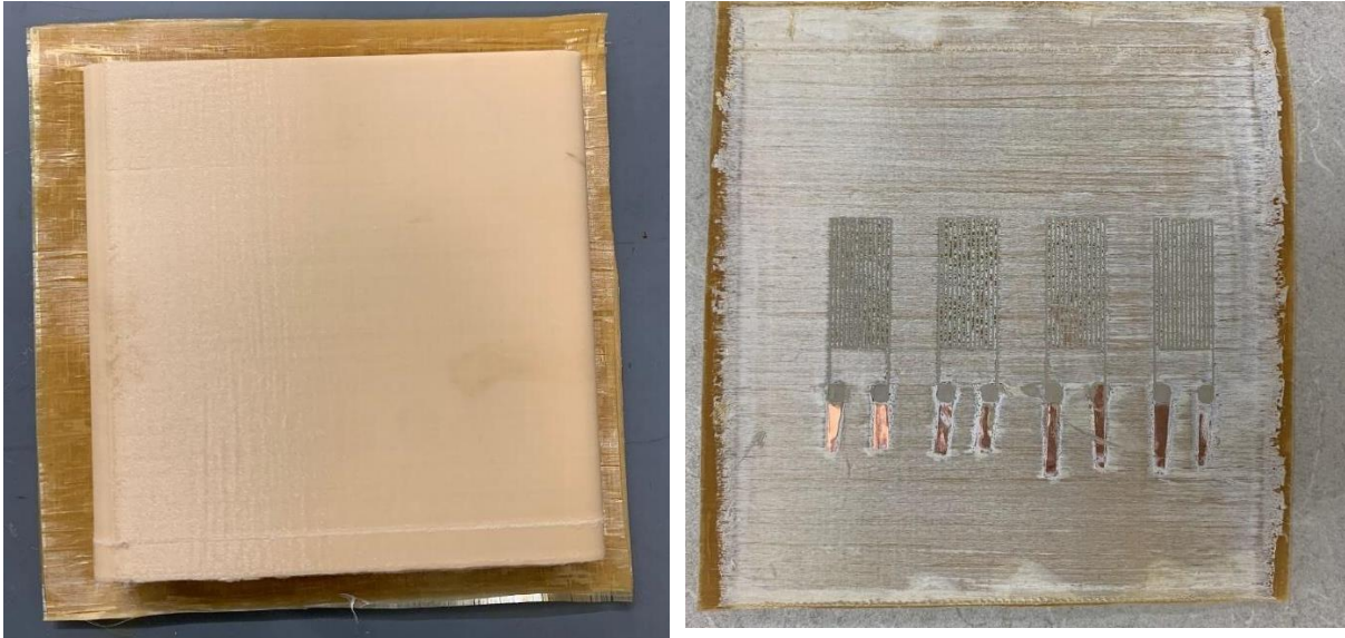
Figure 3.5 PES tooling after curing FRP composite laminate (a) and after tool dissolution in DMSO (b), showing the successful transfer of the printed strain gauges from the surface of the PES tooling to the FRP composite surface.
