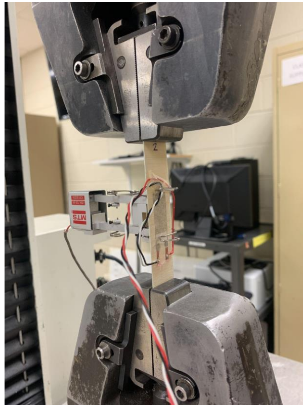
Figure 3.8 Test configuration for tension testing including an extensometer to measure strain.
