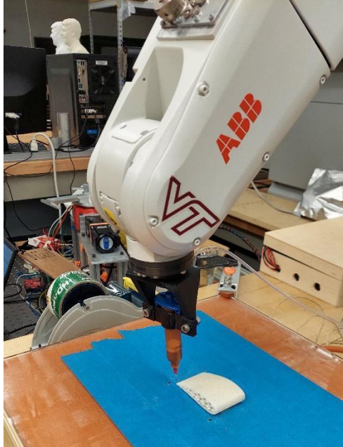
Figure 2.3 Conformal DIW of Dupont CB-028 onto airfoil tool via 6-axis robotic arm.
