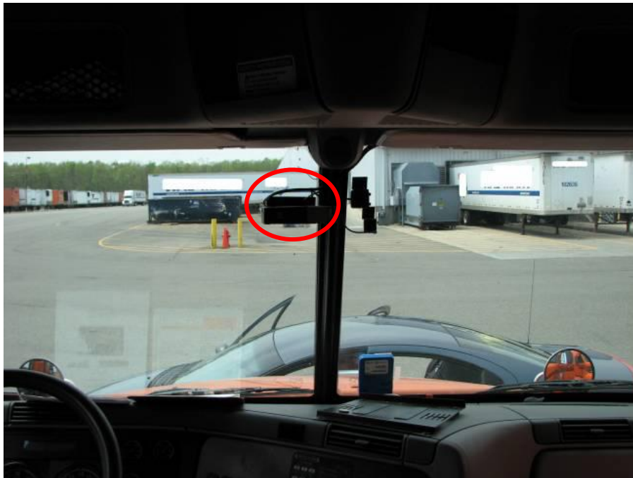
Figure 5. Face camera located in truck cab (Blanco et al., in press, p. 13). Used with permission of Dr. Blanco.
