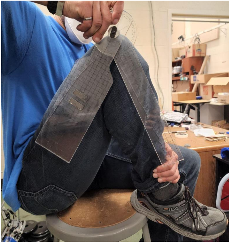
Figure 6.2: Range of Motion measurements, method two (Knee Flexion)
