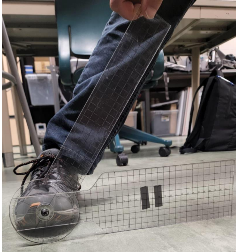
Figure 6.4: Range of Motion measurements, method two (Ankle Inversion)
