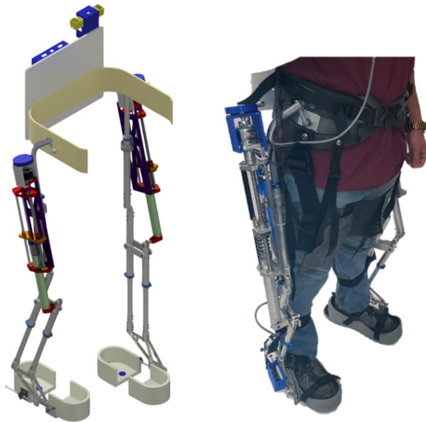
Figure 2.1: Orthographic view of CAD model and real-world underactuated exoskeleton
