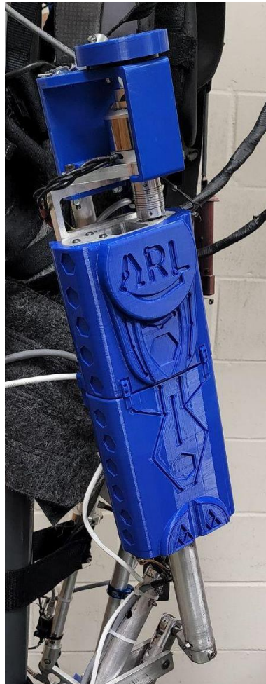
Figure 4.2: Exoskeleton actuator safety cover
