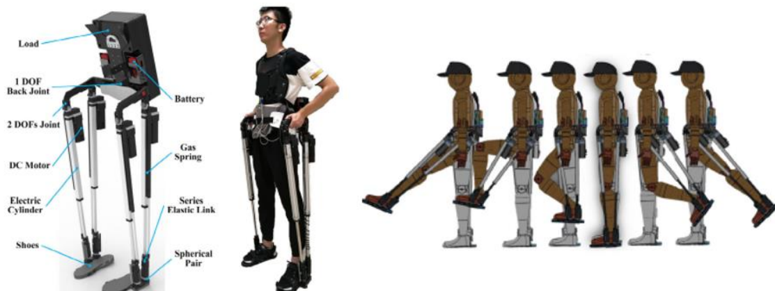
Figure 1.2: PALExo labeled diagram and gait model
