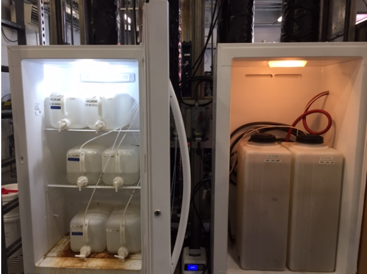
Figure 2: Image of refrigerated 20 gallon influent and 5 gallon influent and effluent sample containers.
