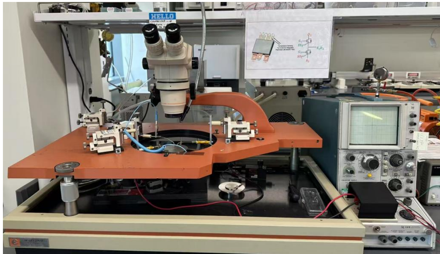
Fig. 11 Probe station and the curve tracer for electrical test.
