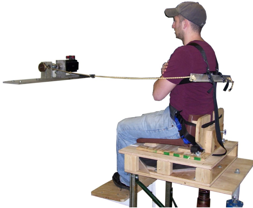
Figure 1: Experimental set-up for anteriorly-directed forces applied to the trunk. A servo motor with torque cell and pulley provided controlled force levels applied to the subject via a chest harness and cable system.
