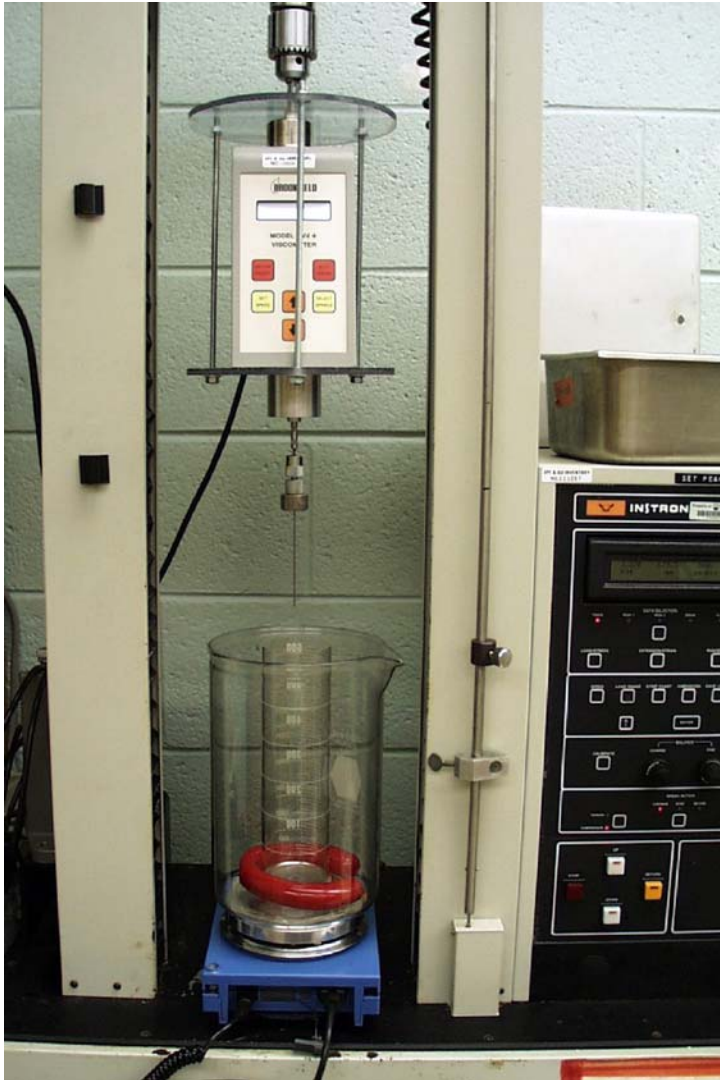
Figure 2. Apparatus for measuring apparent viscosity of melted Mozzarella cheese. A Brookfield Viscometer with t-bar spindle has been attached to an Instron Universal Testing Instrument.
