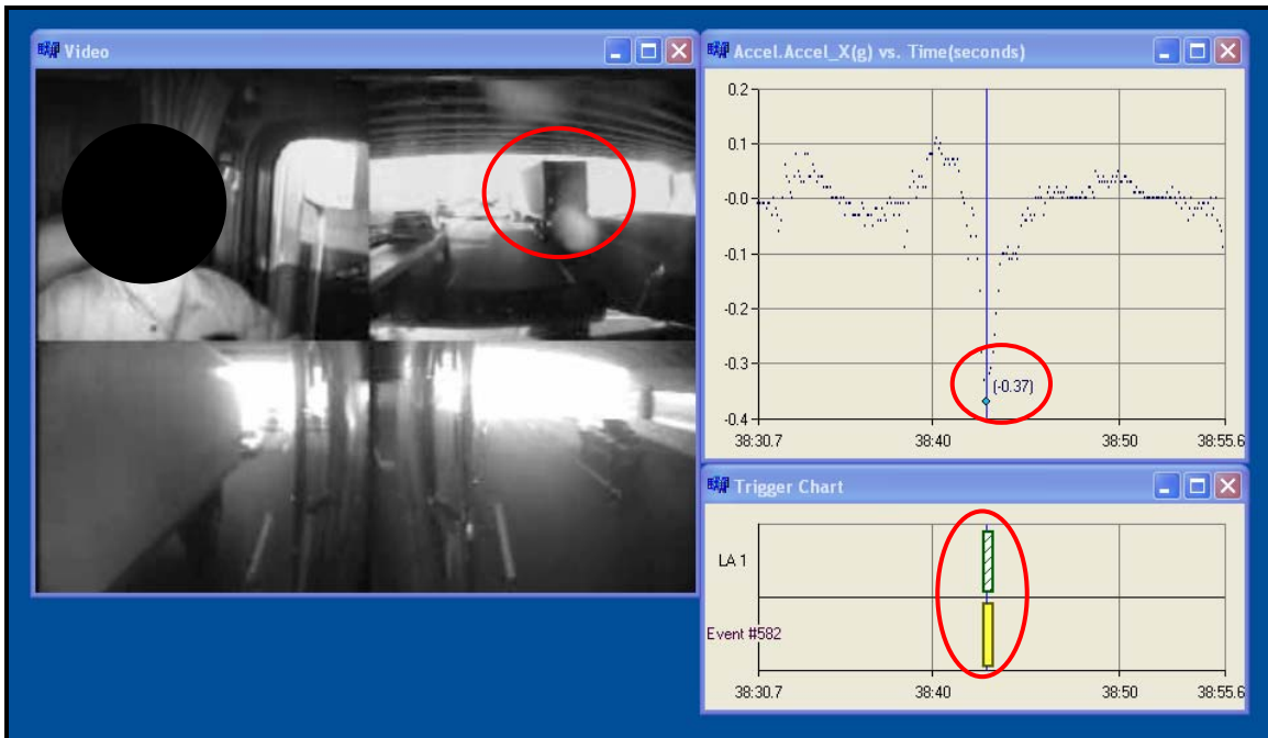
Figure 10. Example of a validated trigger where the LA was less than the pre-set value of |0.35g| .
