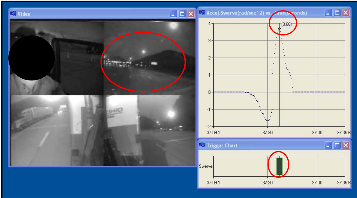
Figure 11. Example of a non-conflict event (with a valid trigger) where the driver’s swerve (quick steering) value was 3.68 (trigger set to \geq 3 ).
