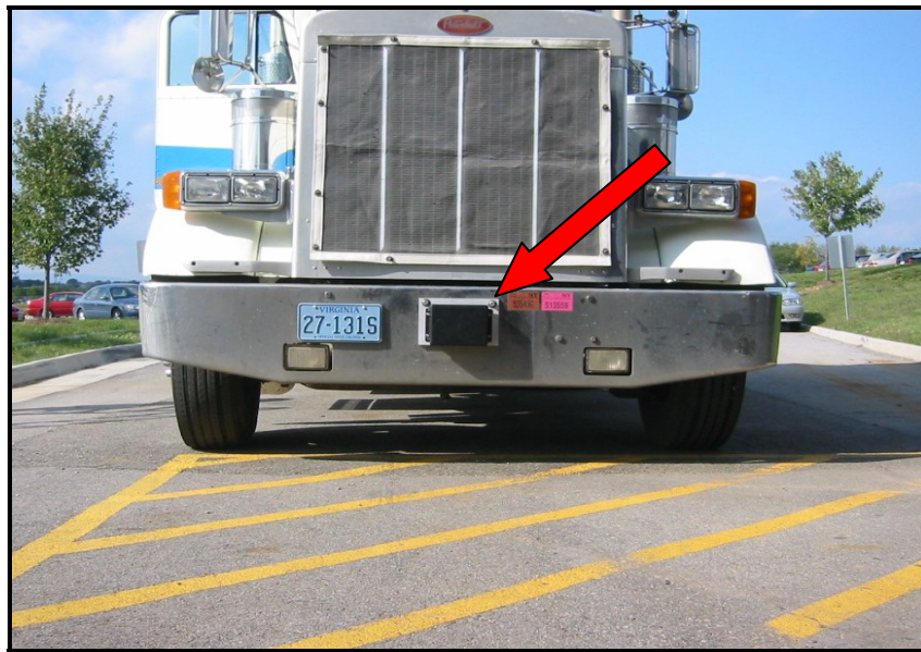
Figure 6. VORAD unit on the front of the truck.
