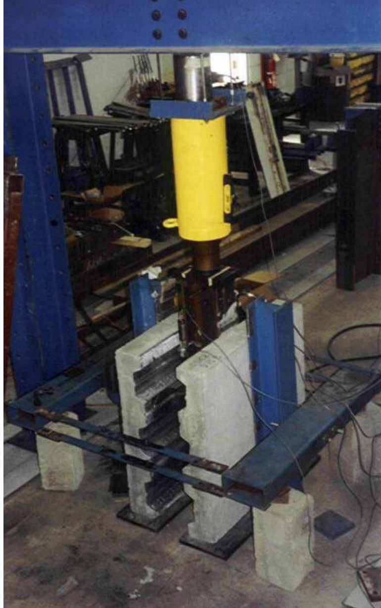
Fig. 1.3 Push-Out Test of a Composite Slab with Formed Steel Deck
