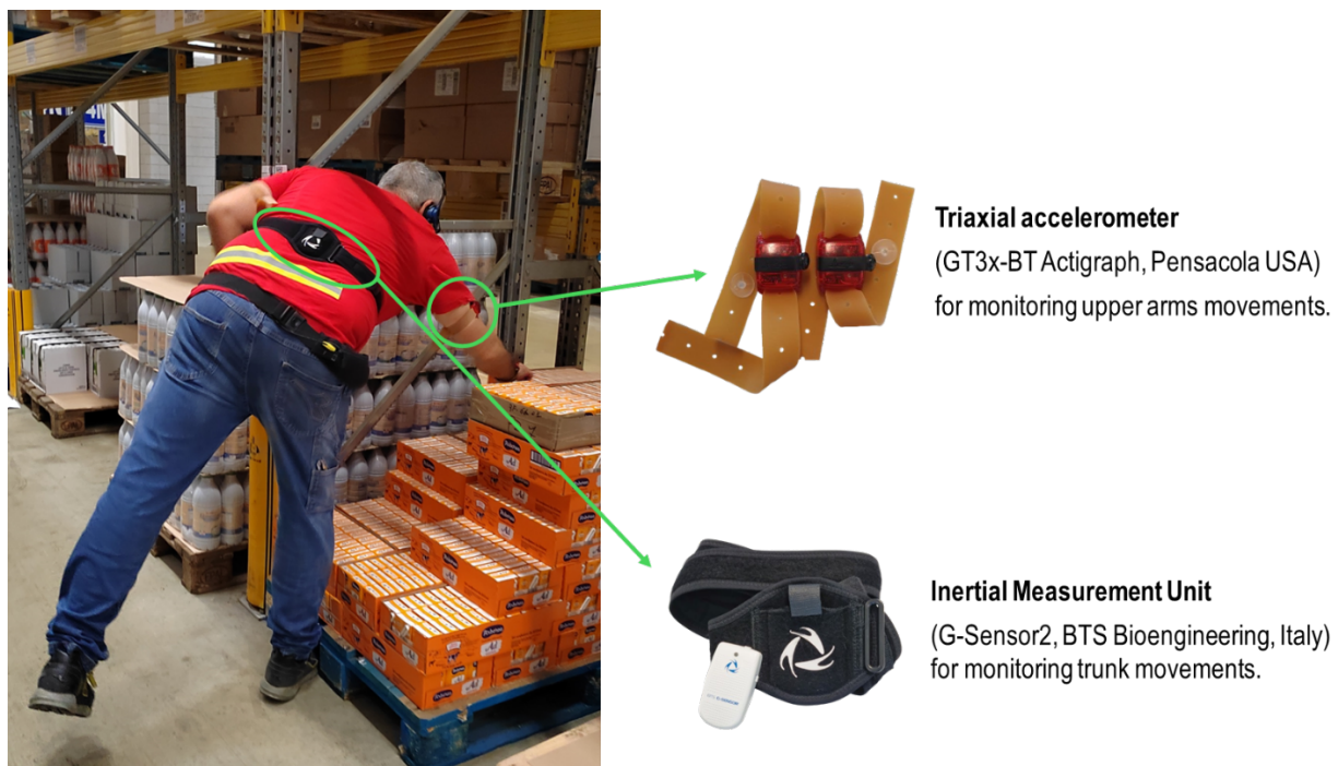
Figure 1: Example of sensor placements. See text for details.
