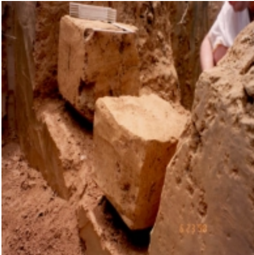
(c) Block sample excavation almost complete.
