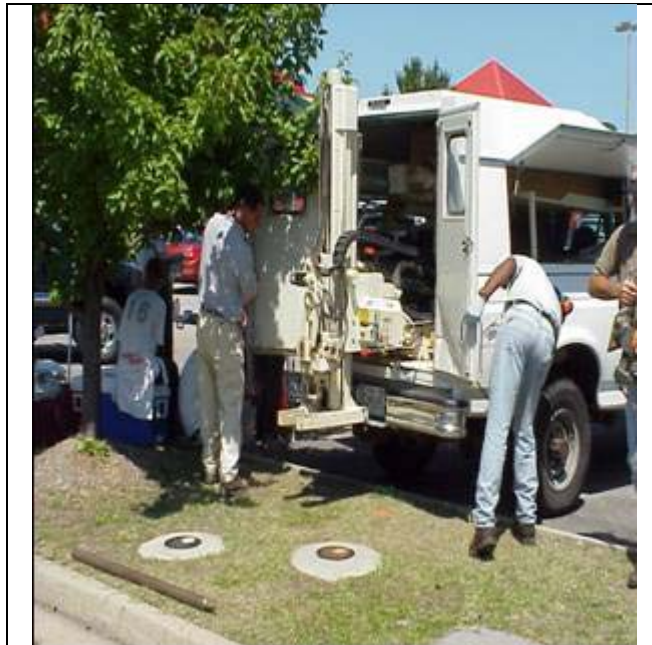
Figure 2-2. Geoprobe™ Drill Equipped with a Hollow Stem Sampling Probe at the Sediment Collection Point. This collection point is located at multilevel sampler 12.
