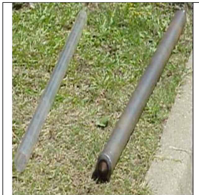
Figure 2-3. Acetate Liner (left) and Hollow-Stem Sampling Probe (right) used for Sediment Collection
