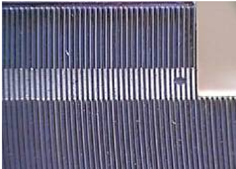
Figure C.2: Finished “Uncracked” Crack Lap Shear Specimen
