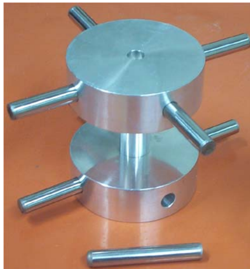
Figure 4.2: The alignment blocks and spacers controlled adhesive thickness and alignment.
