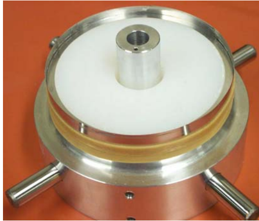
Figure 4.3: Picture of half of a napkin-ring specimen ready for adhesive to be dispensed.
