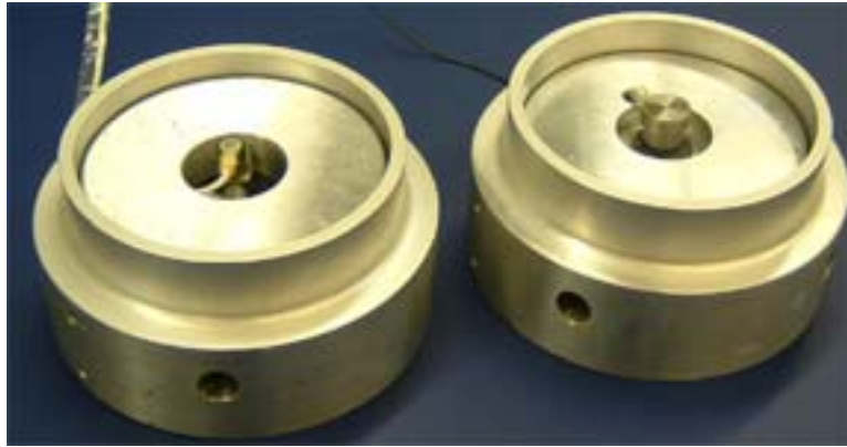
Figure 4.6: A Capacitec model HPB-75 was used to measure the axial deformations
