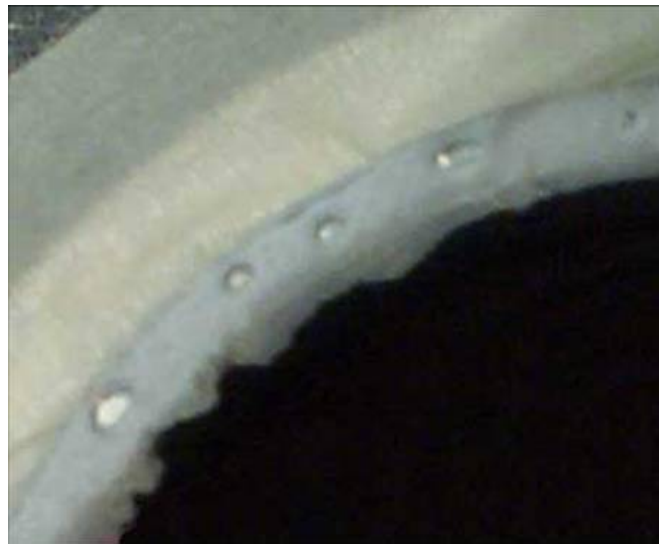
Figure 4.12: Picture of a failed napkin-ring specimen with voids.
