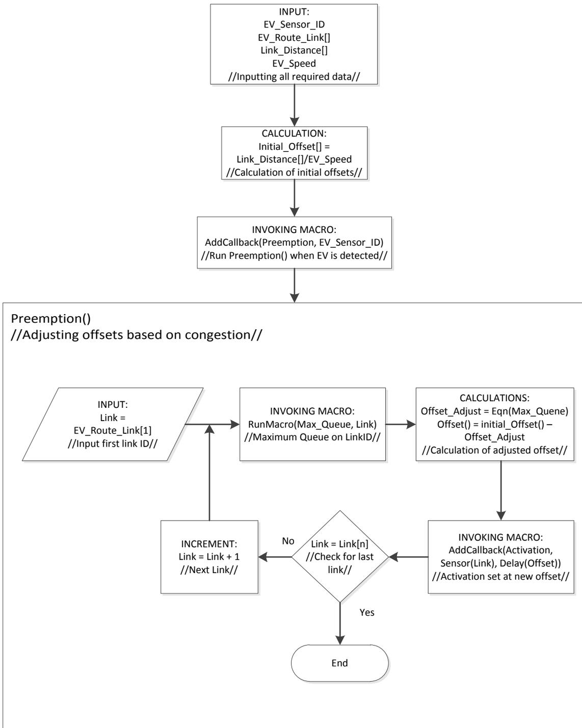
Figure 9- Logic for simultaneous offset adjustment algorithm
