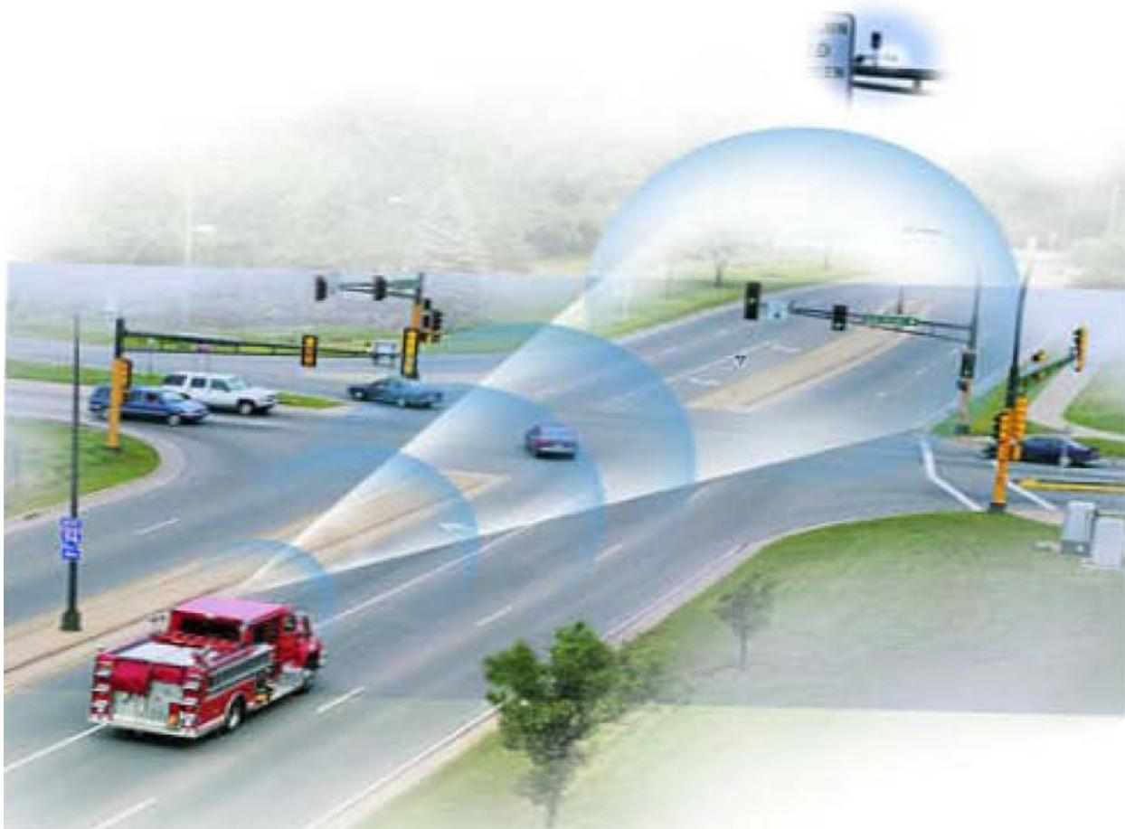
Figure 3 - Emergency vehicle detection and preemption at an intersection [2]
