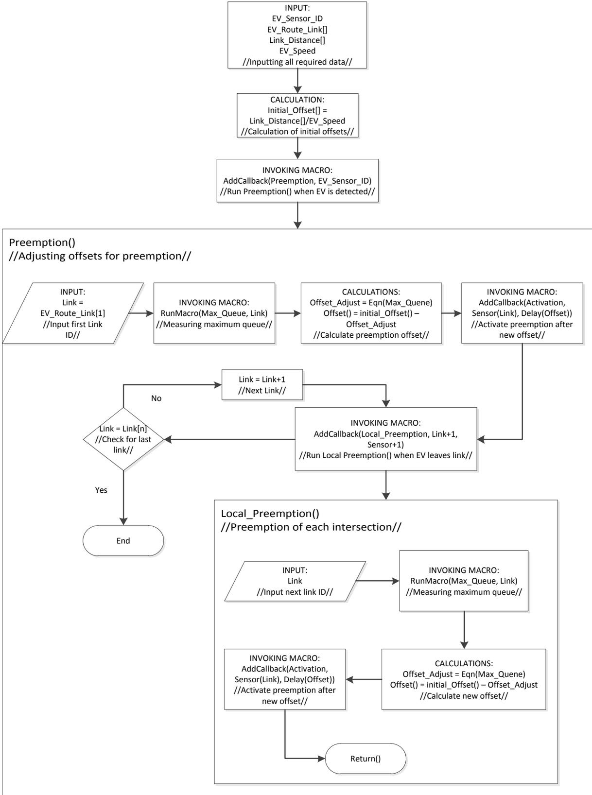
Figure 10 - Logic for progressive offset-adjustment algorithm
