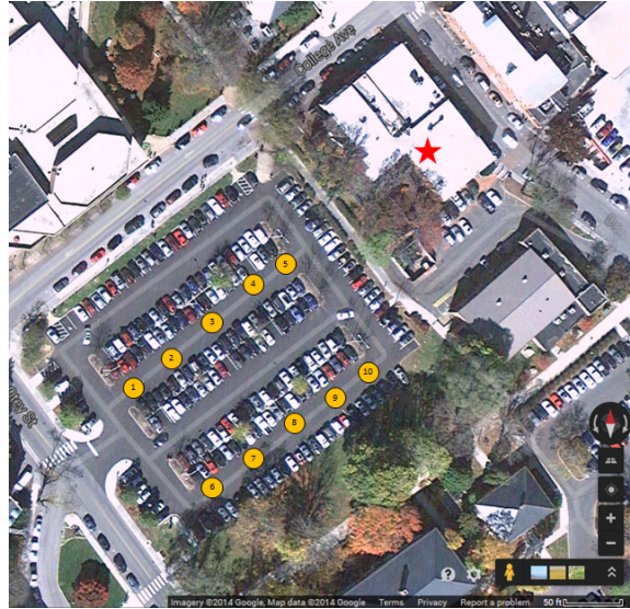
Figure 5.10: WiFi Scanner's Locations around Squires Building Parking Lot. The Red Star is the Location of the WiFi Router Being Tested.
