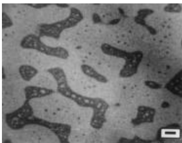
Figure 6-12. TEM image of RuO 4 stained thin sections of 25 wt % 15 K poly(arylene ether sulfone) modified cyanate ester network. 19
