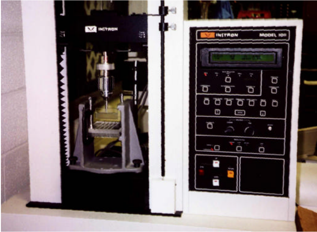
Fig. 3. Instron with plexiglass tooth attachment used for testing noodle firmness.
