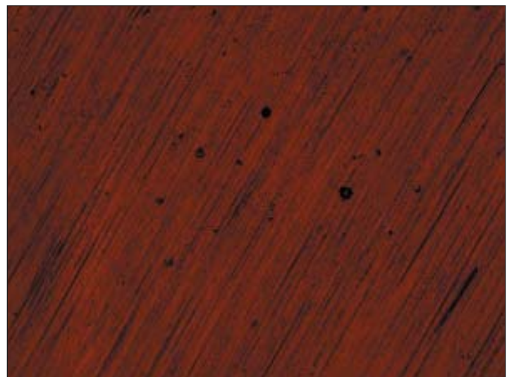
Figure 8. Micrograph of Pyrowear 675 in 30% Seawater after 1 week, taken with Zeiss microscope
