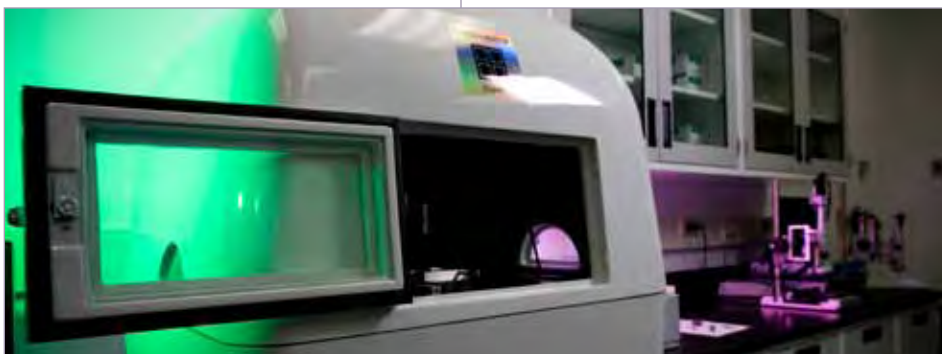
This TribolIndenter, used for measuring the hardness and elastic modulus of thin films and coatings, is just one of the devices used in ICTAS-sponsored research.
