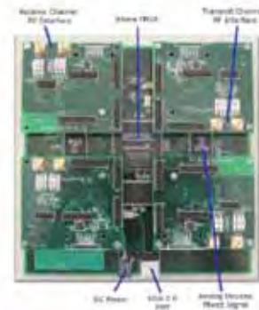
Figure 3. A single CR node consists of a small PC and a USRP RF front end.
