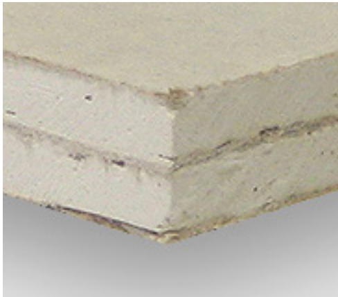
Quiet Rock Quiet Rock is made of a viscoelastic material sandwiched between two gypsum layers. The gypsum board has the mass to block sound waves, while the viscoelastic material damps the wave vibrations.
