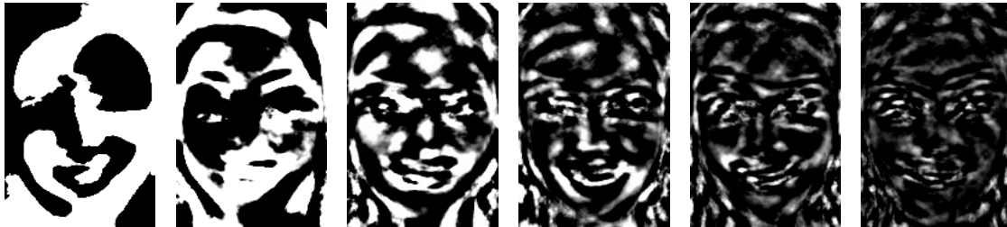
Figure 4.3: Images of different eigenfaces. From left to right, images represented by the 10th, 50th, 100th, 150th, 200th and 250th eigenface, respectively.
