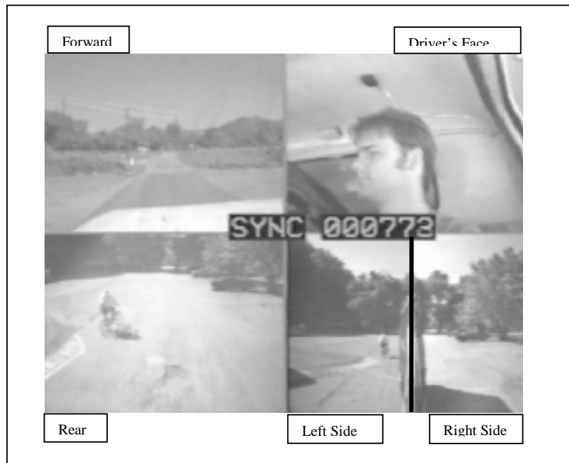
Figure 10. Split-screen presentation of the five camera views. Driver shown is a hardware technician at Virginia Tech.
