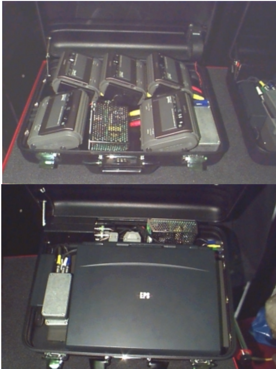
Figure 8. One of the black box data collection systems that were installed in L/SH trucks.
