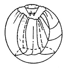
Figure 4. Cone and slice fracture pattern in an impacted sphere (after Gildemeister and Schonert, 1972).
