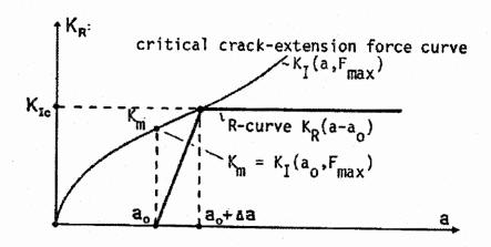
Figure 16. Simple bilinear R-curve and critical stress intensity factor curve (after Ouchterlony, 1983)
