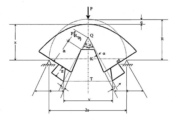
Figure 22. Kinetics of semi-circular fracture model (after Karfakis, et al., 1986)
