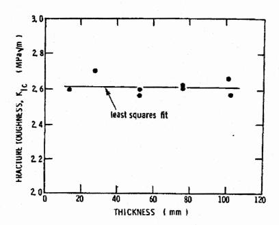
Figure 13. Effect of specimen thickness on fractrue toughness of Westerly granite (after Schmidt and Lutz, 1979).
