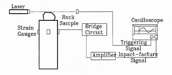
Figure 6. Schematic representation of ULCD test set-up (after King et al., 1991)
