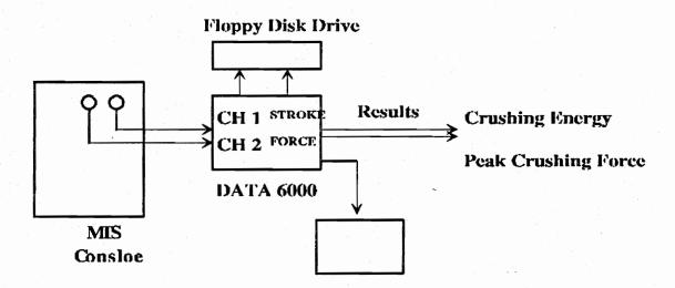
Figure 25. Schematics of HECT and data acquisition system
