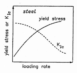
Figure 10. Effect of loading rate on fracture toughness and yield stress of metals at constant temperarure (after Shah, 1987)
