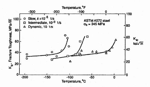
Figure 9. Effect of loading rate on the fracture toughness of ASTM A572 steel (after Dowling, 1993)
