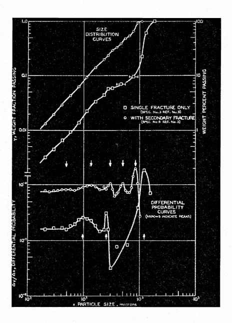
Figure 1. Size distribution and differential probability curves for two glass spheres by single fracture (in geltin) and with secondary fracture (in steel retaining ring) respectively.
