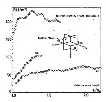
Figure 15. Fracture energy consumption rate R for Indiana limestone (after Ouchterlony, 1983)
