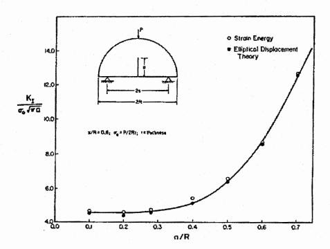
Figure 20. Mode I stress intensity factor for SCB specimen (after Chong et al., 1987)
