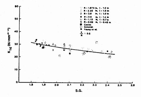
Fig 21. Fracture toughness versus specific gravity using average of stress intensity factor, compliance and J-integral methods (after Chong et al., 1987)
