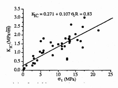
Figure 8. Correlation of mode I fracture toughness with uniaxial tensile strength (after Whittaker et al., 1992)
