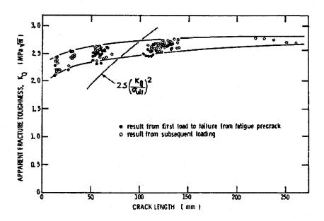
Figure 12. Apparent fracture toughness of Westerly granite versus crack length for all compact specimens (after Schmidt and Lutz, 1979).
