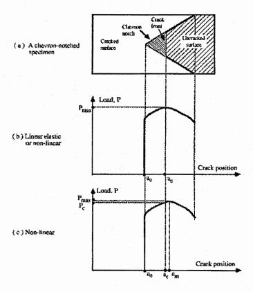
Figure 18. Chevron notch and load-crack front relationship (after Whittaker, 1992)
