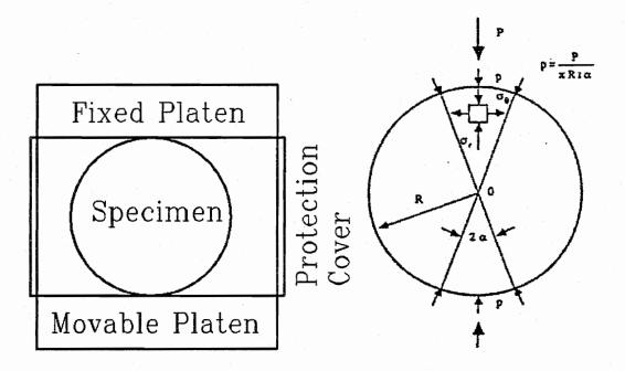
Figure 23. Cylindrical specimen under diametrical compression and its theoretical background
