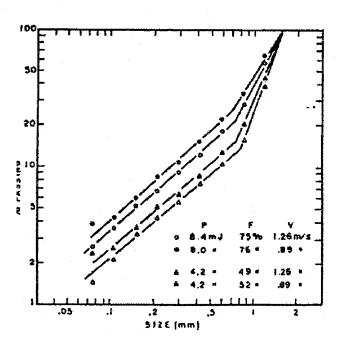
Figure 2. Size distribution of calcite at two energy levels and two impact velocities (P is the input energy level, F is the breakage probability and V is the impact velocity) (after Krough, 1978)
