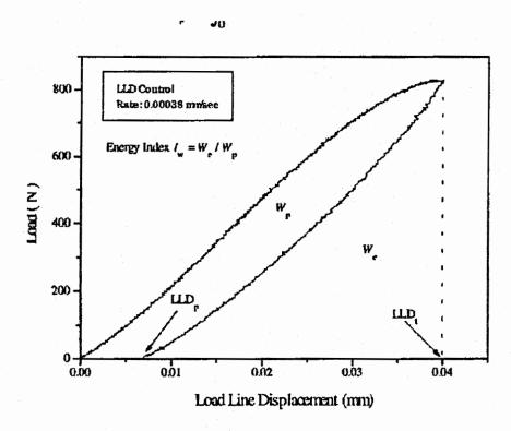
Figure 5. Energy index determination (after Karfakis, 1991)
