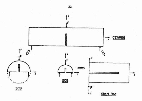
Figure 17. Complete fracture toughness characterization from a single core (after Chong et al., 1987)
