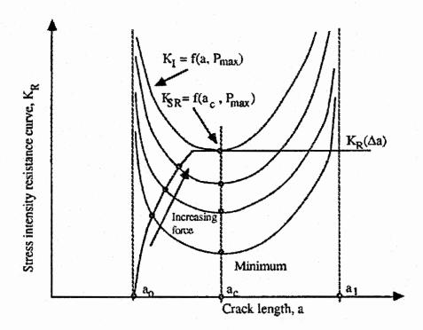
Figure 19. Fracture resistance curves of SR specimen and an assumed R-curve with a flat upper part for determining the point for evaluating fracture toughness (after Ouchterlony, 1982)
