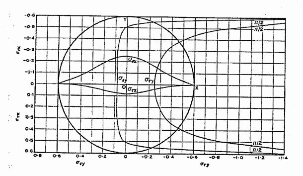
Figure 24. Theoretical stress distribution along the vertical (OY) and horizontal (OX) diameters (after Hondros, 1959)
