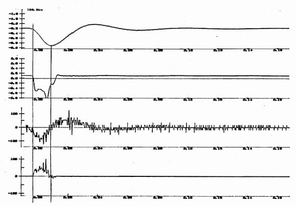
Rock sample: Sandstone, Equipment settings: Stroke = 1", Rate = 99 Hz
