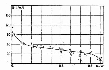
Figure 14. Specific work of fracture  $\overline{R}$  for SENB of Chelmsford granite (after Ouvhterlony, 1983)
