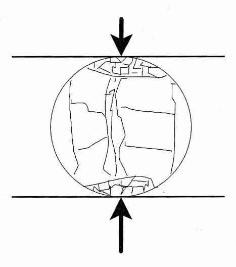
Figure 28. Breakage pattern for cylindrical specimen under impact
