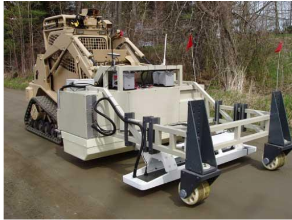
Figure 1.3. Nemesis with a mine detection sensor suite.
