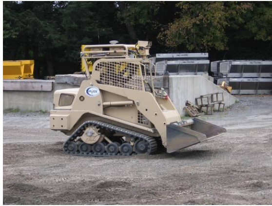
Figure 1.1. ARA Nemesis Platform. An ASV RC-60 base vehicle.
