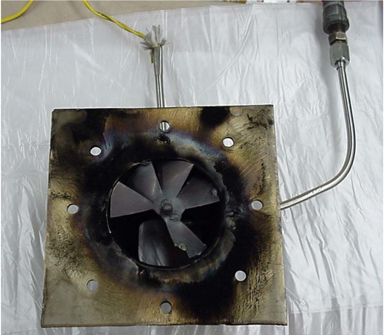
Figure 3.1: Lower combustion chamber after test
