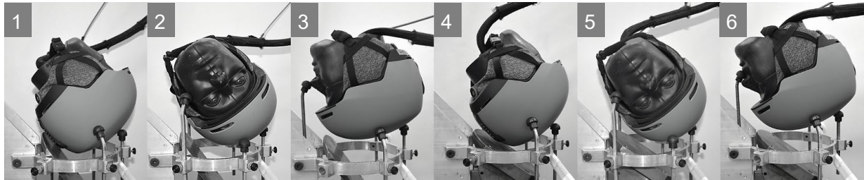
Figure 2. Six impact configurations. Configurations 1, 2, and 3 are tested on a higher anvil angle (55°) and represent impacts with a higher tangential component. Configurations 4, 5, and 6 are tested on a lower anvil angle (35°) and represent impacts with a higher normal component.
