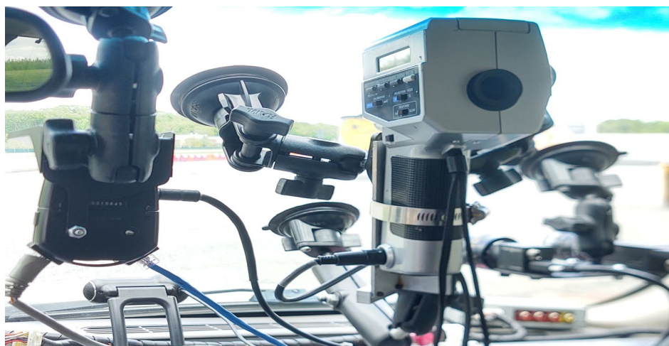
Figure 7. Photo. REIMS components behind windshield.
