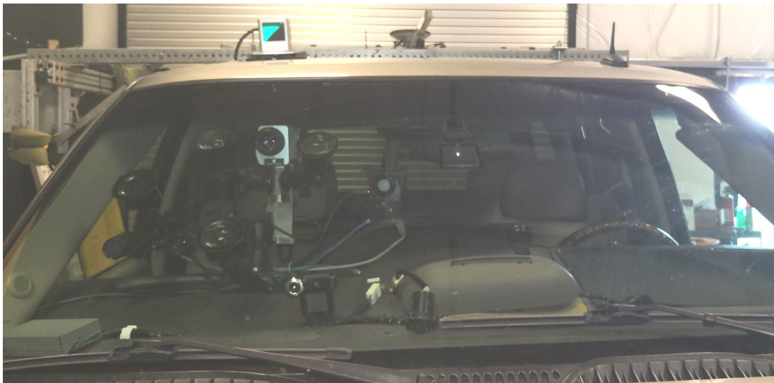
Figure 6. Photo. REIMS components – front view.
