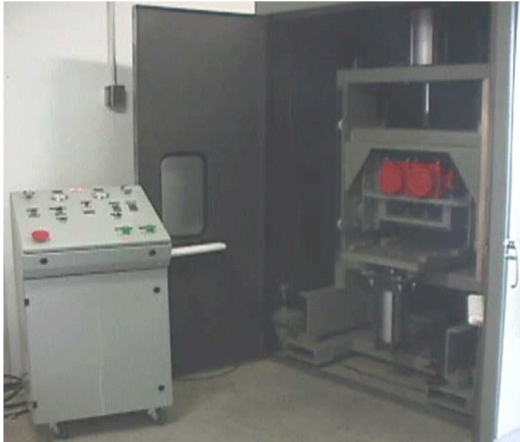
Figure 3.1 PTI Vibratory compactor (photo by author).
