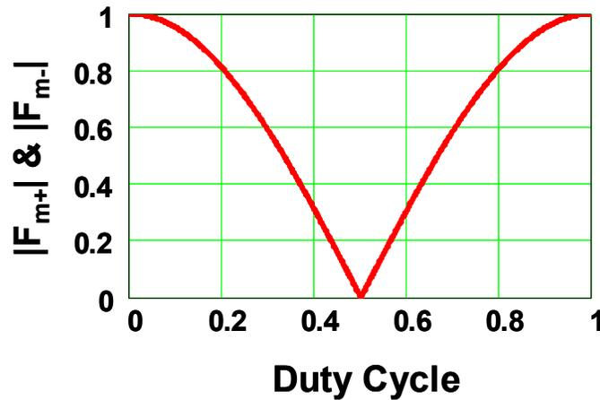
Figure A.3. Magnitude of  $F_{m+}$  and  $F_{m-}$  as a function of the duty cycle for the double-edge modulation.
