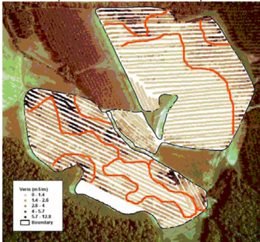
Figure 1. Soil EC Data from Veris 3100 with management zones delineated in orange
