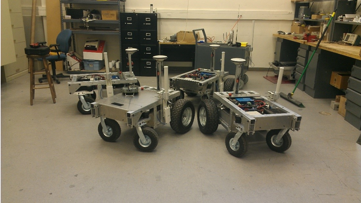
Figure 4.1: Differential drive test platforms (TURTLEs).
