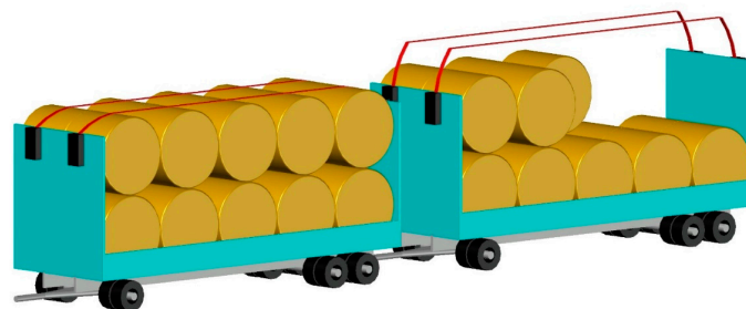
Figure 2. Concept for adaptation of ALSS for tandem trailers, identified as ALSS-2.
