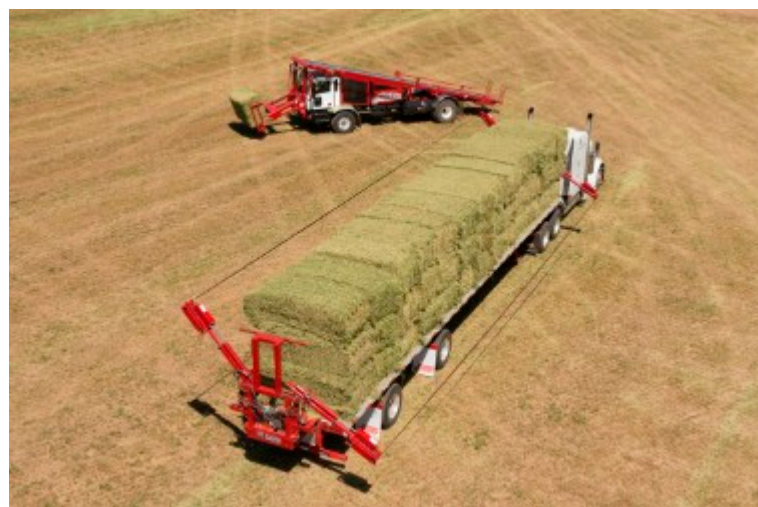
Figure 1. Load of large rectangular bales ( 1\text{ m} \times 1.2\text{ m} \times 2.4\text{ m} ) secured with Stinger ALSS. (Photo reprinted with permission from Stinger Incorporated.).
